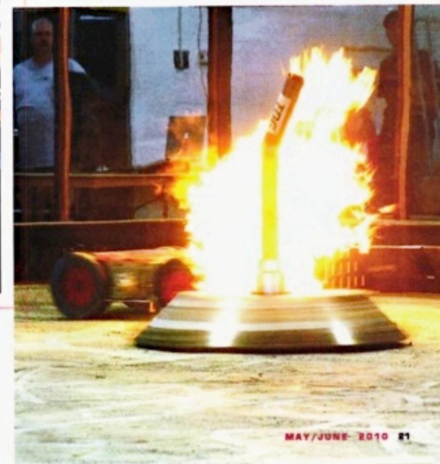
These are the big boys: the 340-pound class. Of that weight, Ziggy is 120 pounds of titanium and delivers over 7,000 pounds of explosive thrust through its flipping arm. Sewer Snake has two movable wedges that it uses to attack other bots and to right itself. It gets its name from its entertaining ability to flip itself over and over again. Both teams are regulars at RoboGames.
