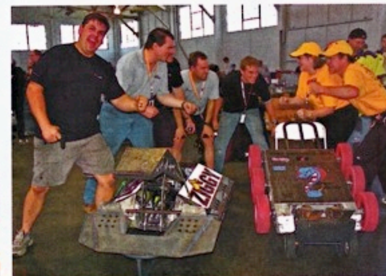
These are the big boys: the 340-pound class. Of that weight, Ziggy is 120 pounds of titanium and delivers over 7,000 pounds of explosive thrust through its flipping arm. Sewer Snake has two movable wedges that it uses to attack other bots and to right itself. It gets its name from its entertaining ability to flip itself over and over again. Both teams are regulars at RoboGames.
